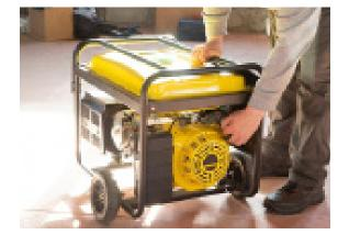
• Make sure equipment has 3-4 feet of clear space on all sides and above it to ensure adequate ventilation.
